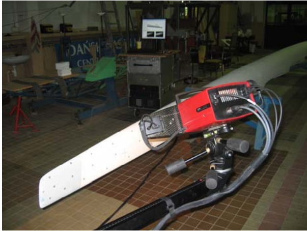
Figure 6 The digital scanning of the hulls, carried out using an ATOS II scanner (CTO S.A., 2007)
